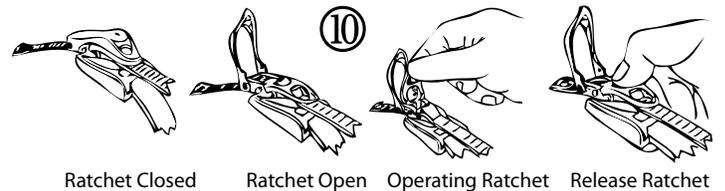
Open cover on ratchet and push button to release the ratchet strap enough to fit XLR Tow Mirror on to existing mirror. Operate ratchet adjuster until snug (10). On larger vehicles additional strap length may be required. The rubber strap on the XLR ratchet adjuster can be adjusted by sliding the quick connect clip lower on the rubber strap (8).
